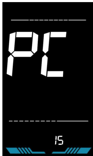
Figure 6-12 Controller current limit setting interface
